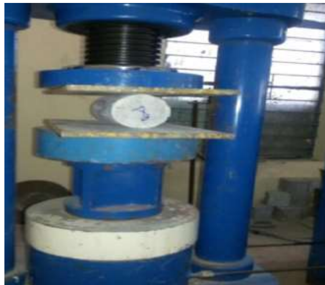
Plate 5: split tensile strength on cylinder
