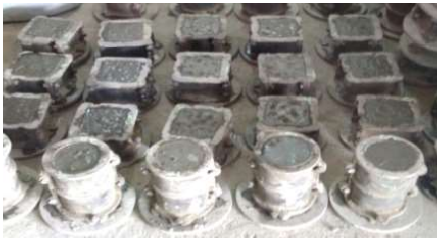
Plate 2: casting of specimens
